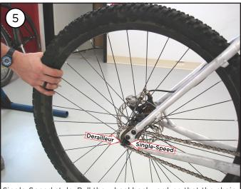
Single-Speed style: Pull the wheel backward, so that the chain is properly tensioned.
